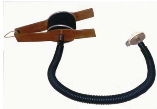
Hand operated bellows and breathing tube and expiratory valve as assembled in 1960 by Dr. Muallem for patient transport
