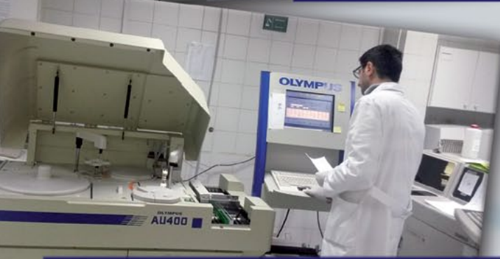
Olympus AU400: a fully automated chemistry analyzer for routine, STAT, urine and homogenous immuno assays
