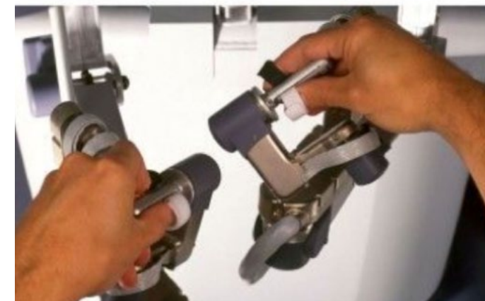
Picture 2 - Translations of the surgeon's movements into robotic arms movements
