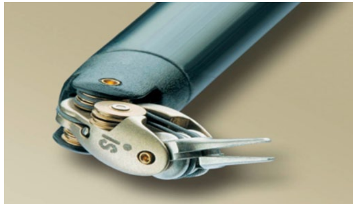
Picture 4 - Endowrist function of the 8mm robotic instruments
